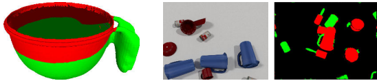
Fig. 3. Left: Task-constraint labels for a bowl and the pour task, where red means grasp away from the bowl opening. Middle and right: synthetically generated image and labels.
