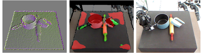
Fig. 1. Grasping for a transport task. Left: Depth gradient, input to the CNN. Middle: the green overlay indicates task-compatible regions encoded by the CNN (here: grasp handles only). Right: Planning and executing a 7DOF grasp (pose and preshape) within a compatible region.
